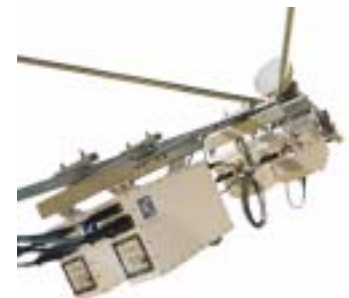
5700 transceivers antenna mounted in 1:1 configuration
