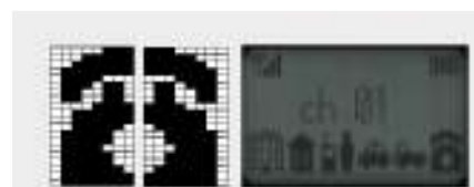
8x20 dot character can be made on a PC and plural characters can be combined on LCD.
